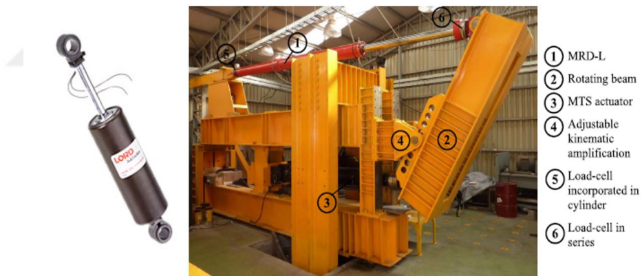
Figure 2.8. RD 1005-3 MRD (Produced by LORD Corp.) and the long-stroke MRD (Source: Zemp et al. (2016))
