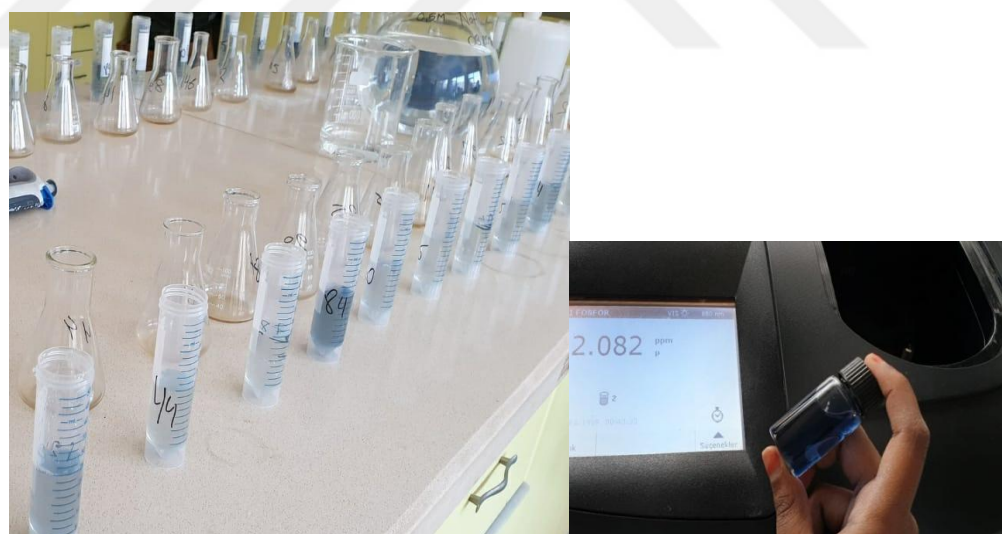
Figure 3.10 Apparatuses used for the analysis of the phosphorus content
