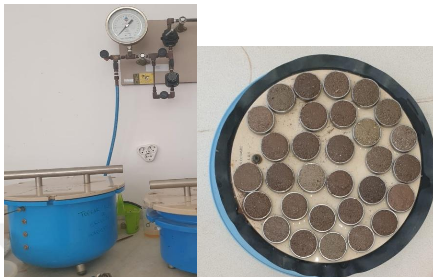
Figure 3.9 The pressure chamber and pressure plate used in measurement of field capacity and wilting point
