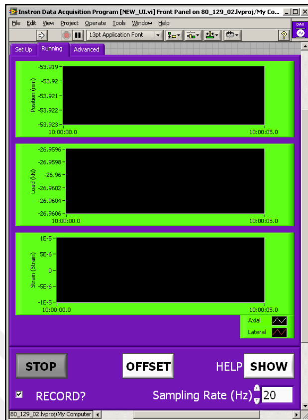
Figure 3.2 Three reading channels for load, axial/lateral strain and position
