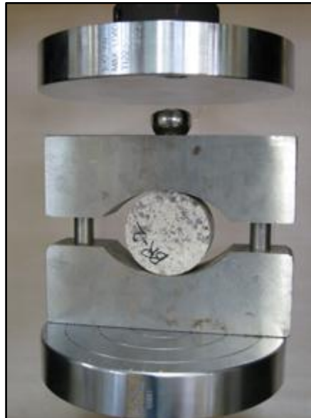
Figure 4.3 Brisbane tuff disc sample between standard Brazilian jaws
