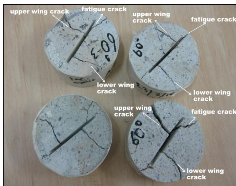
Figure 7.37 \beta = 60^\circ inclined notch and newly formed crack patterns on CCNBD specimens tested under diametral compressive cyclic loading
