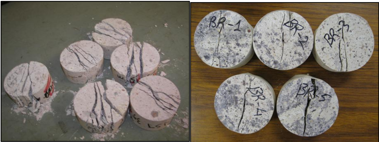
Figure 4.8 Failed Brisbane tuff specimens (a) NST35 and (b) NST207 under standard Brazilian jaws
