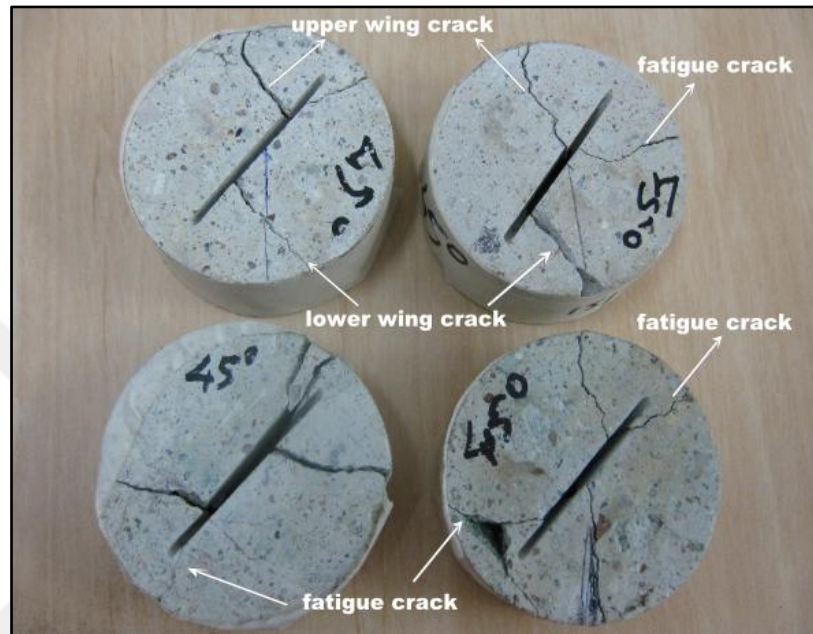
Figure 7.33 \beta = 45^\circ inclined notch and newly formed crack patterns on CCNBD specimens tested under diametral compressive cyclic loading
