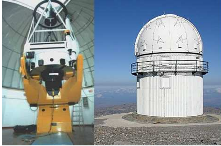
Figure 4.1. A photograph of 1.3 m cassegrain focus telescope of the Skinakas Observatory, Crete, Greece
