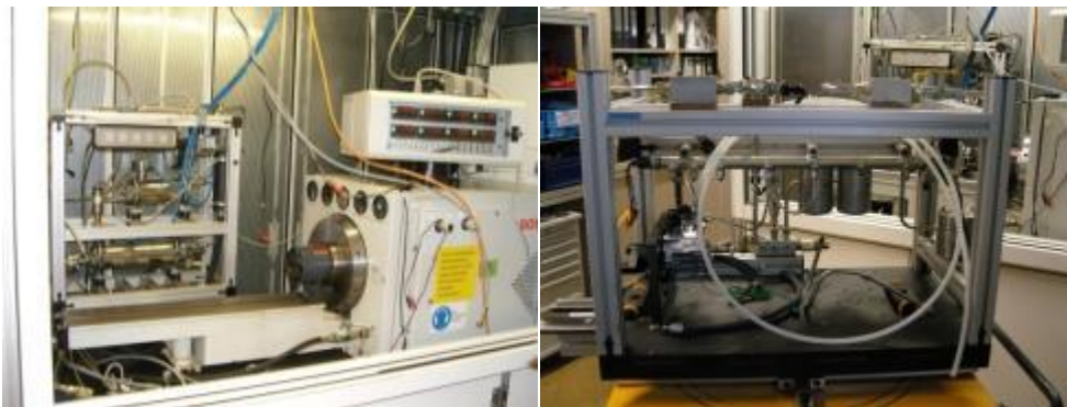
Figure 5.28 : Fuel injection pump rig test [10].
