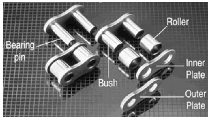
Figure 4.4 : Sub-components of timing chain [11].
