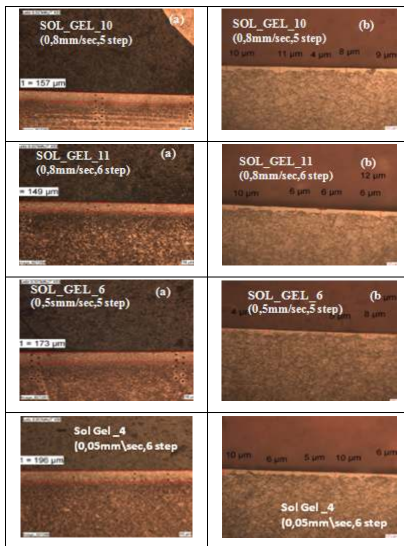
Figure 7.12: a) Thickness of the compound layer of Sol-Gel \text{TiO}_2 coated samples with different dipping speeds and coating steps (etched with Nital)(X500) b) Thickness of the diffusion layer of Sol-Gel \text{TiO}_2 coated samples (etched with Adler) (X50)
