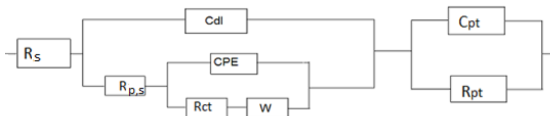
Figure 4.84 : Equivalent circuit diagram of PCz. (R(C(R(Q(RW))))(CR) [Chi squared: 4.984 \cdot 10^{-4} , n = 0,6627 , Monomer: 5 \cdot 10^{-2} M Cz, Method: PD at 2 cycles, 50 mV/s, Electrolyte: 0,1 M ACN/ Bu 4 NClO 4 , WE: Pt (button electrode), RE: Ag/AgCl, CE: Pt (wire)]
