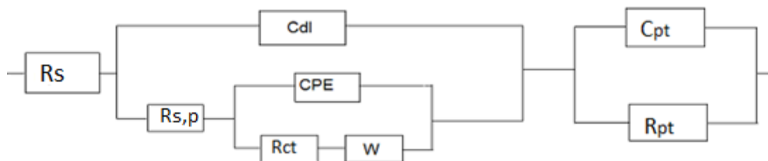
Figure. 4.125 : The equivalent circuit diagram of PIN. [Chi squared: 4.534 \cdot 10^{-4} n: 0.6008 . Monomer: 0,1M IN, Method: PD at 2 cycles, 50 mV/s, Electrolyte: 0,1 M ACN/ NaClO 4 , WE: Pt (button electrode), RE: Ag/AgCl, CE: Pt (wire)]
