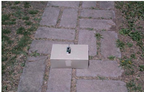
Figure 4.4.a Magnetic sensor is located under the sunlight for studding the effect of temperature variation on AMR sensor
