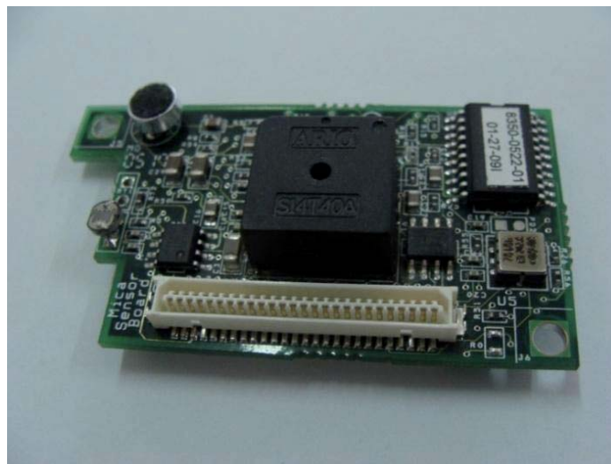
Figure 2.3 MTS310CB sensor board
