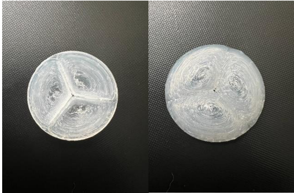
Figure 4.1 Prototype aortic valve scaffold produced with 3D printing
