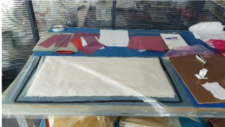
Figure 3.37. Vacuum-bagging of all layers.
