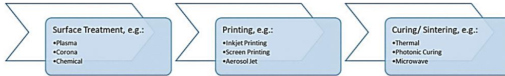
Figure 2.10. Schematic presentation of a printing process including pre-treatment of surface, printing and post-processing [31].
