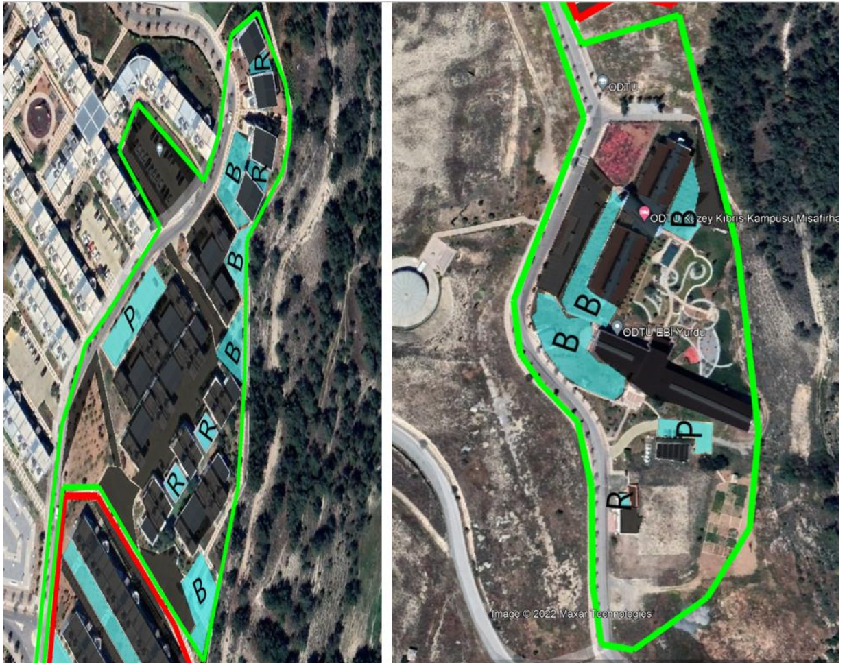
Figure A 1. LID application in Basin 2 (METU-NCC)
