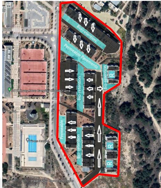
Figure 4.8. Placement of LIDs in Basin 1 (METU-NCC)
