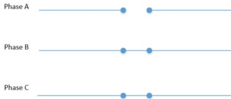
Figure 2. 7. Open conductor fault [33].
