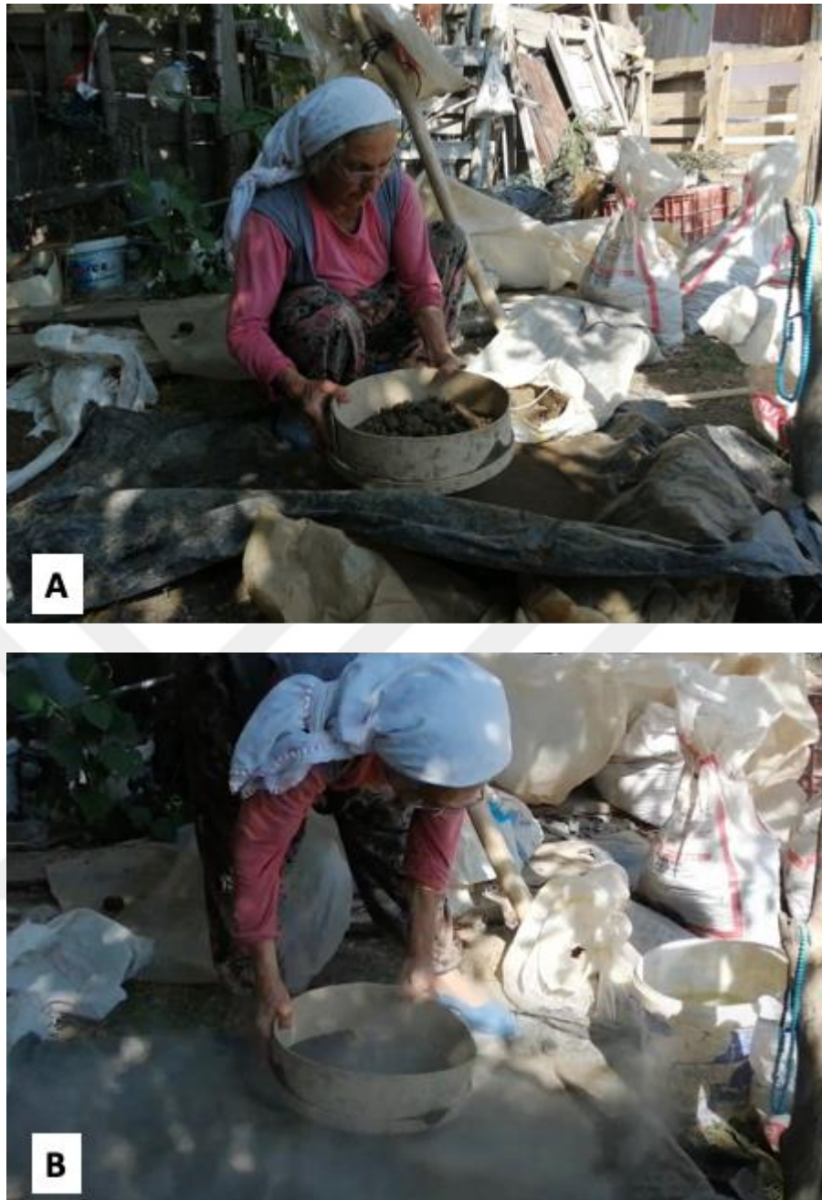
Figure 1.3. Photographs showing the process of sieving A) the Dont clay; the clay aggregates are visible on the top of the sieve B) the additional material
