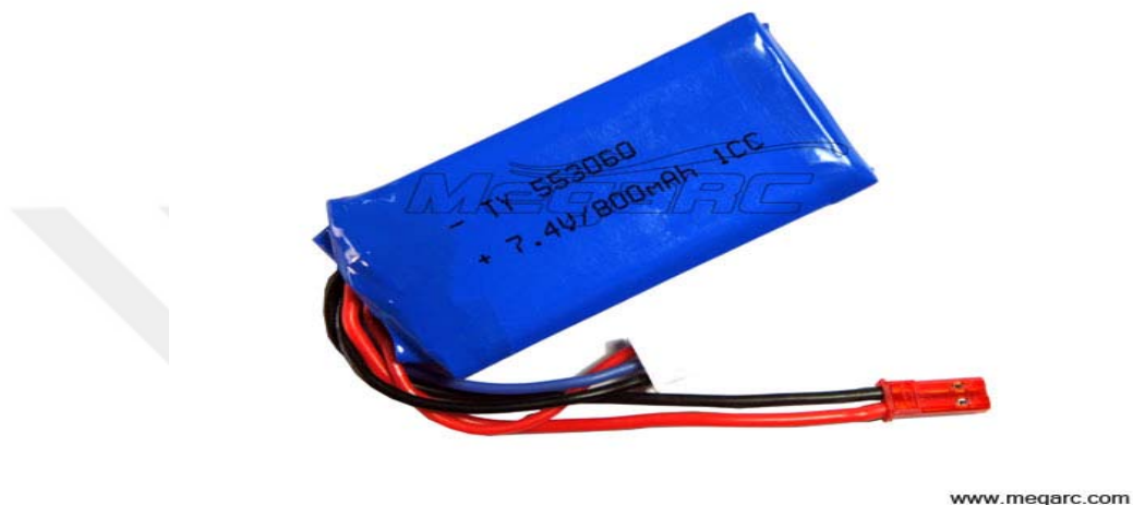
Figure 4.5 A power supply battery of 7.4v
