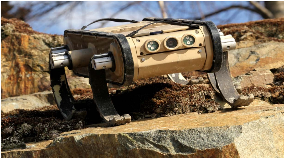
Figure 4.2 Exploration robot called RHEX which has been designed by Boston Dynamics Firm.
