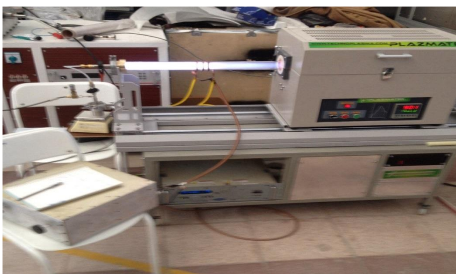
Figure 5.2. By using 250W at the ICP view began to turn on the power before starting graphene synthesis work.
