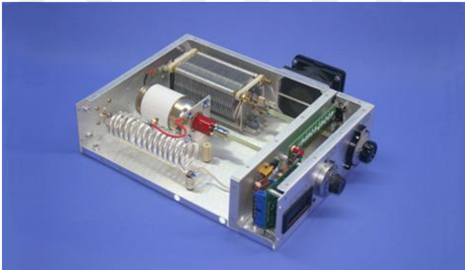
Figure 1.16 Image for matching device. Impedance matching side view of unit (Andrew S., 2012)
