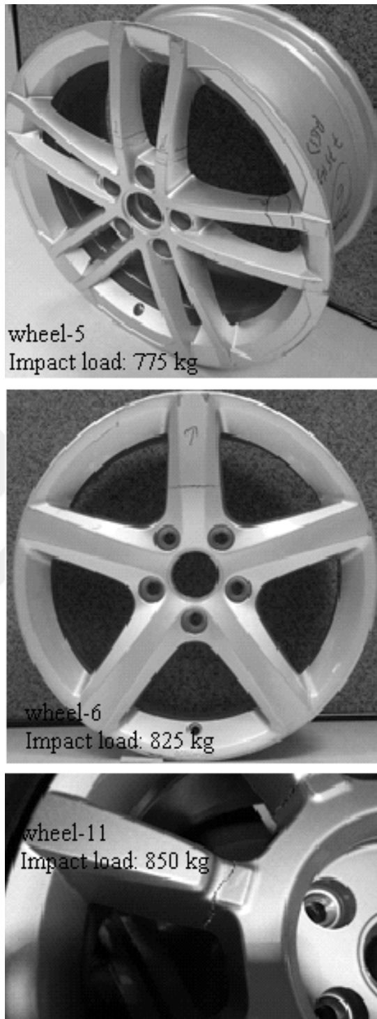
Figure 3.10. Some of the wheels failed in the impact tests
