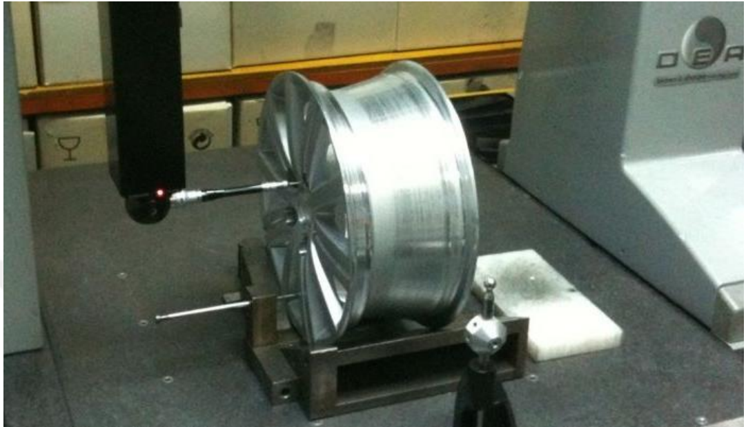
Figure 3.8. Measuring the plastic deformation by CMM
