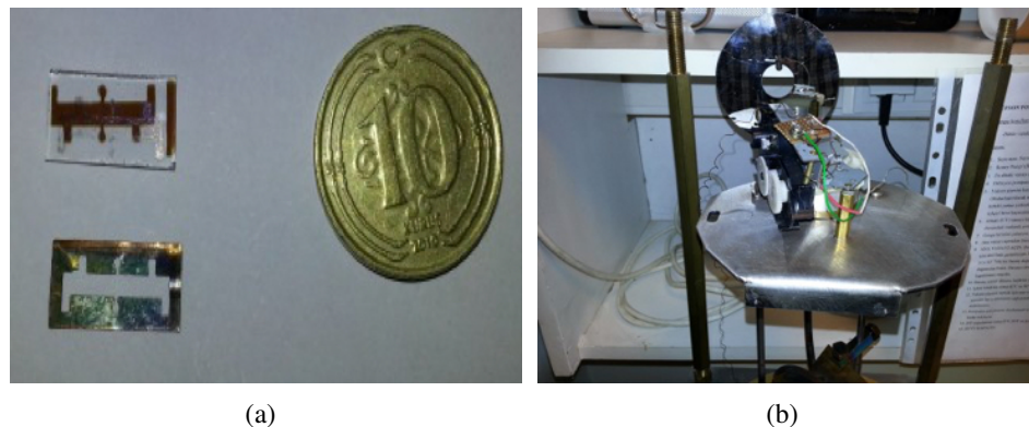
Figure 3.4 : (a) Sample mask and a film on quartz, (b) electrically motorized part.
