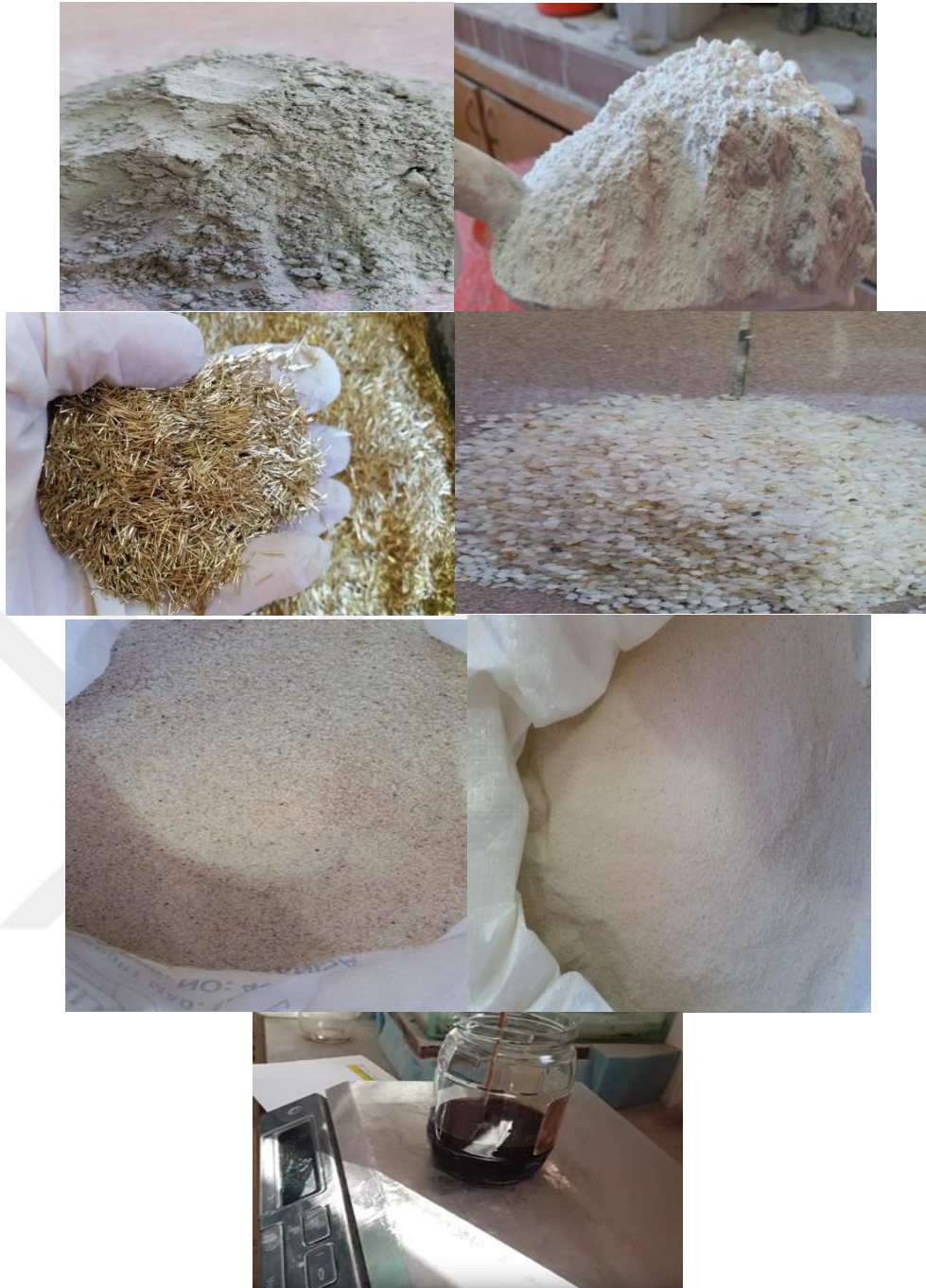
Figure A1 Photographic view of materials used for UHPC production
