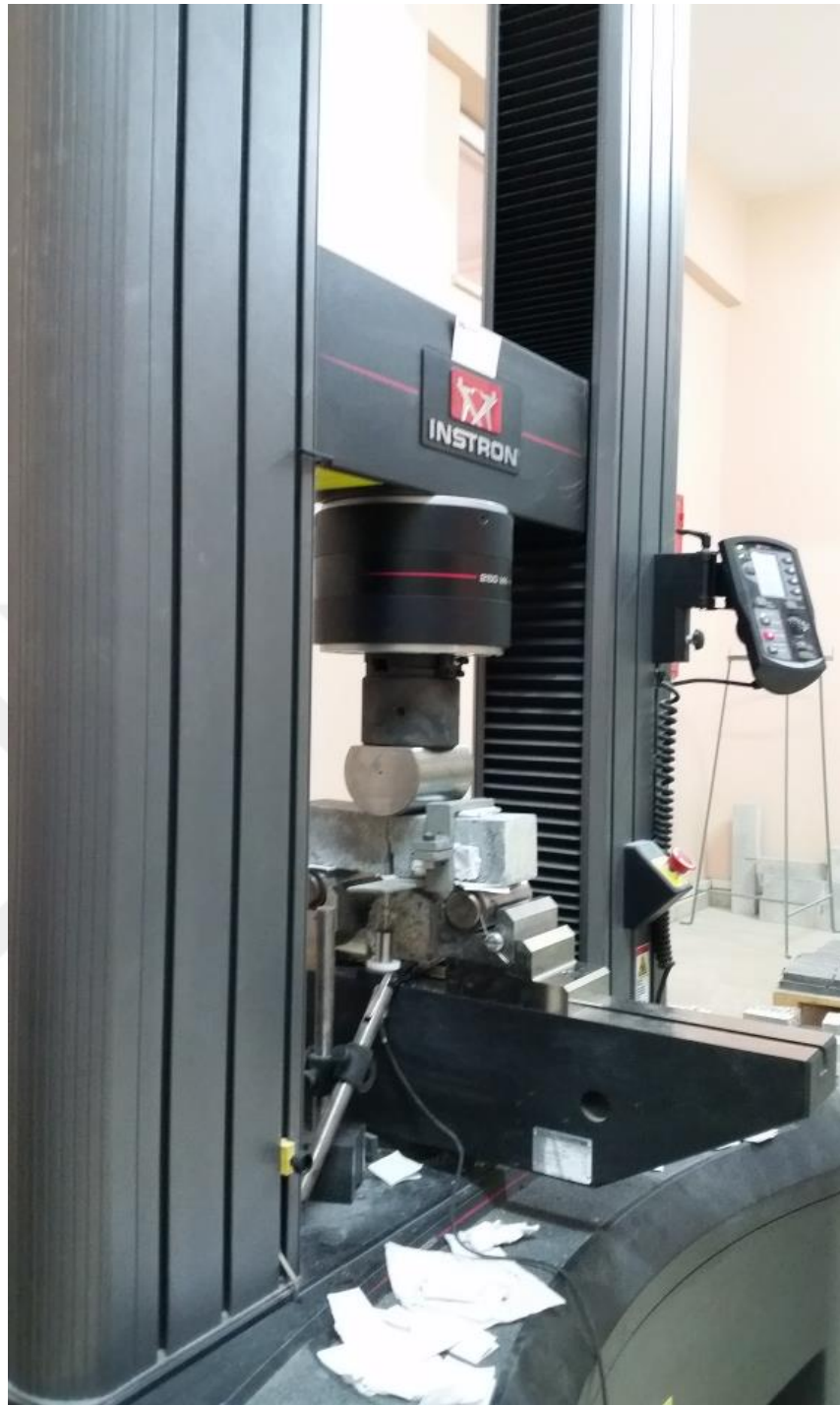
Figure A4 Setting the prisms on the testing machine
