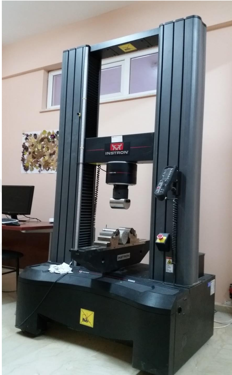
Figure 3.7 Photographic view of universal testing devices and three point flexural testing fixture
