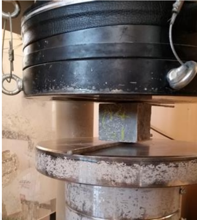
Figure 3.5 Sample during splitting tensile strength
