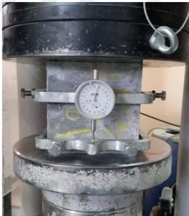
Figure 3.6 Sample during Modulus of elasticity test
