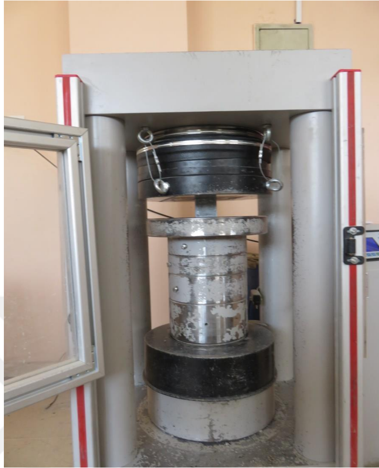
Figure 3.4 Compressive strength instrument with specimen during test
