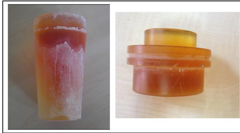
Figure 74 Coupling Material used in test motor firing tests
