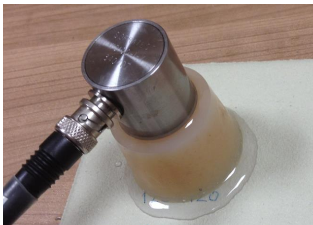
Figure 30 Ultrasonic sensor and BNC connector with coupling material
