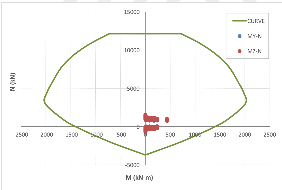
Figure A.20. Q_{10} case pile M-N interaction diagram for Combination 3
