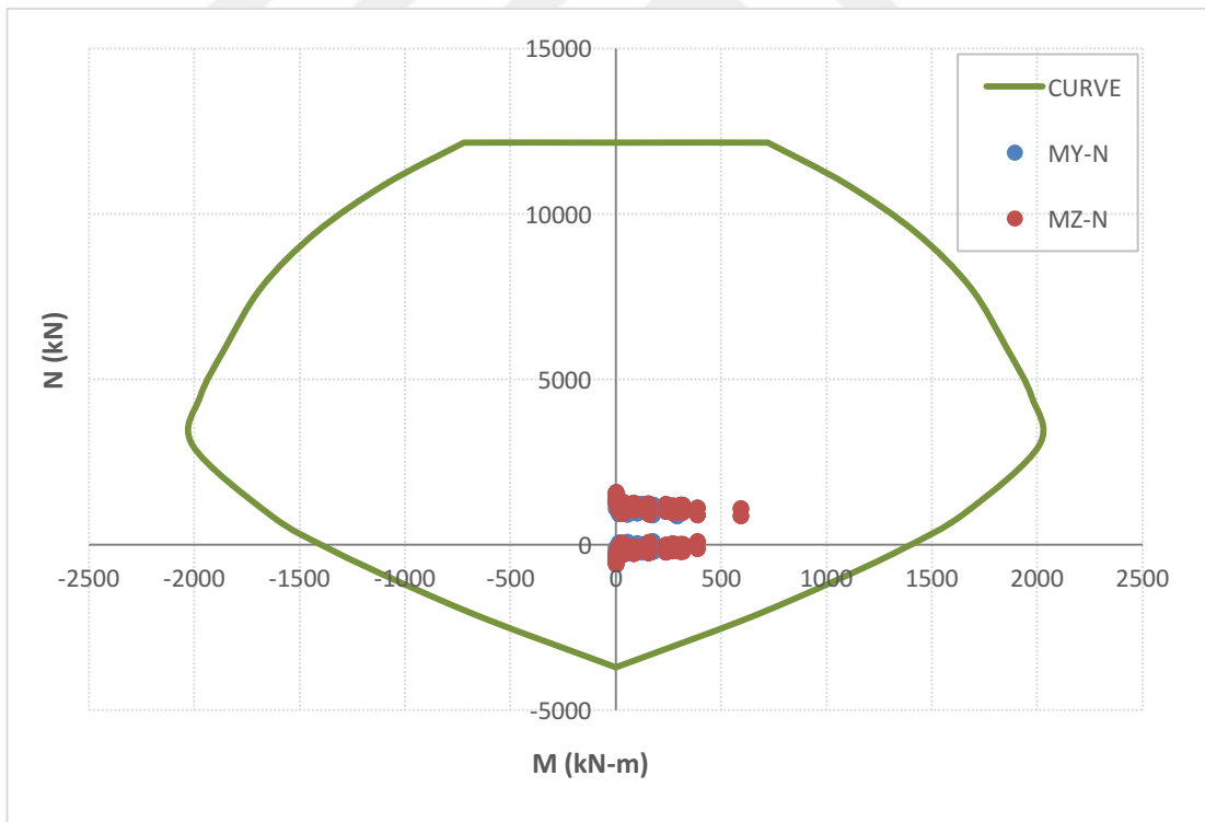
Figure A.34. Q 50 case pile M-N interaction diagram for Combination 5
