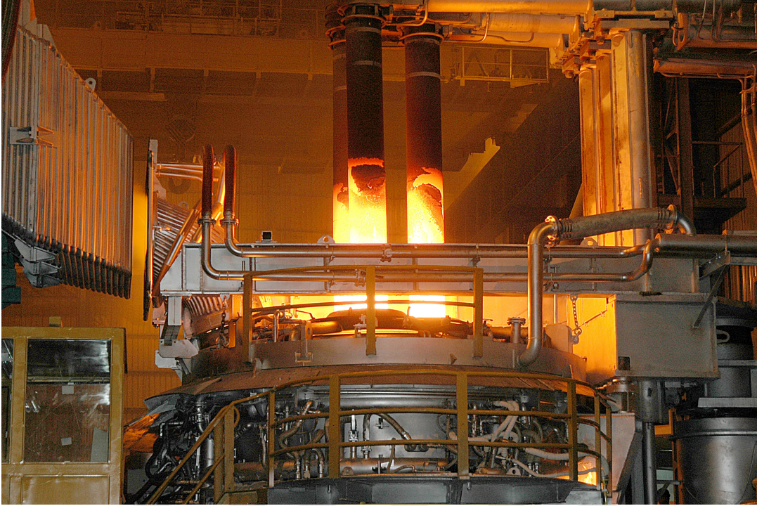
Figure 1.1: A 135-MVA, 135-tonne electric arc furnace, first melting cycle just after commissioning / by courtesy of NURSAN Iron and Steel Inc., Payas, Iskenderun, Turkey.
