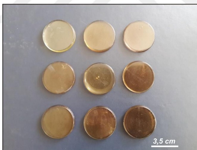
Figure 4.0.5: Pictures of the sample preparation process. Homogeneous glass disks are prepared by using fusion machine.
