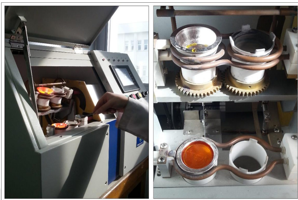
Figure 4.0.4: Fusion machine and glass disk preparation process.
