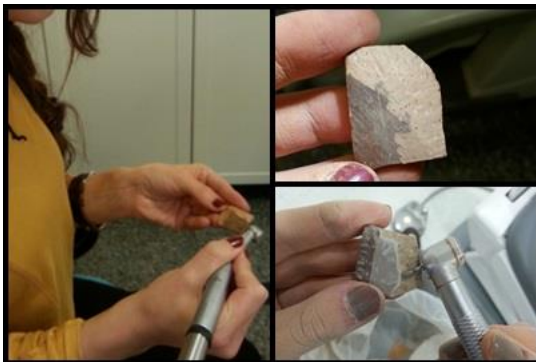
Figure 4.0.2: Image of sample preparation process. Contaminations were removed from internal and external surface of the pottery sherds using diamond coated abrader.
