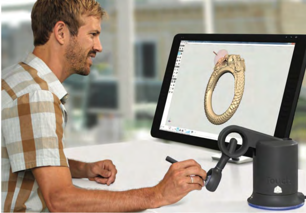
Figure 4.12 Geomagic Touch haptic force-feedback device (“Touch(TM) 3D stylus,” n.d.)
