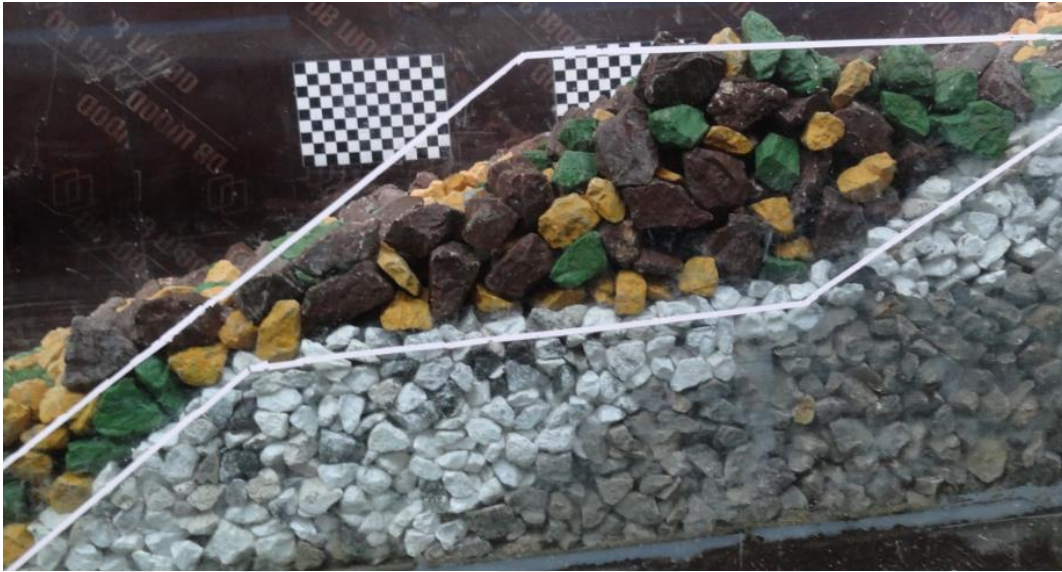
Figure 4.25 View of Section 4 after set 1 (1000 waves)
