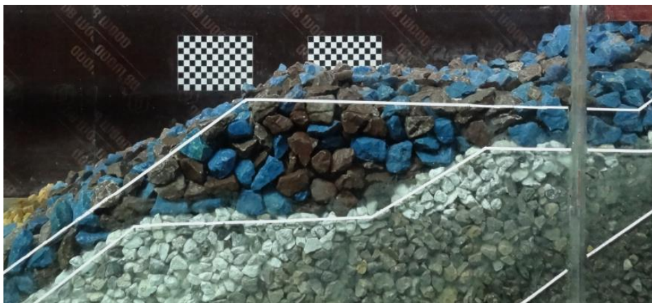
Figure 4.35 View of Section 5 after set 1 (1000 waves)
