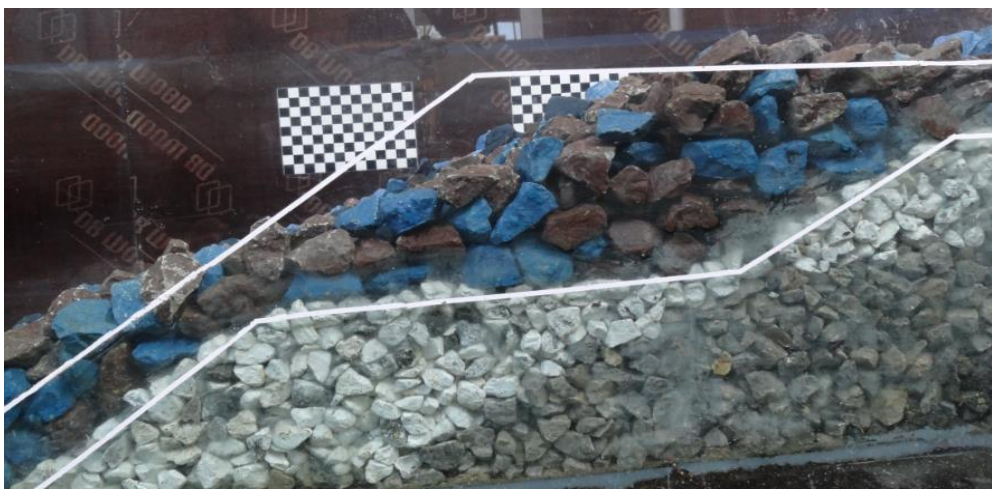
Figure 4.38 View of Section 5 after set 1 (10000 waves)
