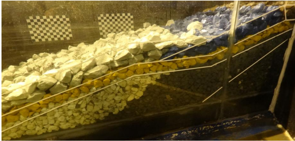
Figure 4.4 View of Section 1 after Set 3 (3000 waves)
