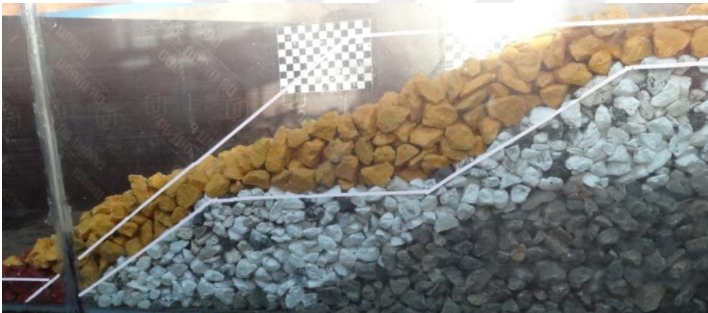
Figure 4.20 View of Section 3 after set 2 (1000 waves)
