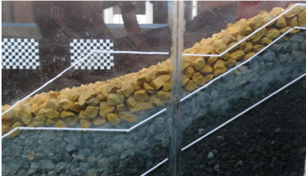
Figure 4.13 View of Section 2 after set 2 (1000 waves)
