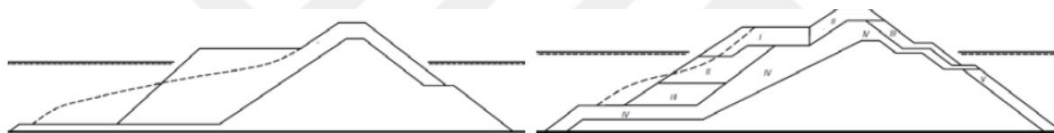
Figure 2.2 Mass armoured and Icelandic-type berm breakwater (dotted line symbolises expected reshaping profile) (Sigurdarson and van der Meer, 2012)
