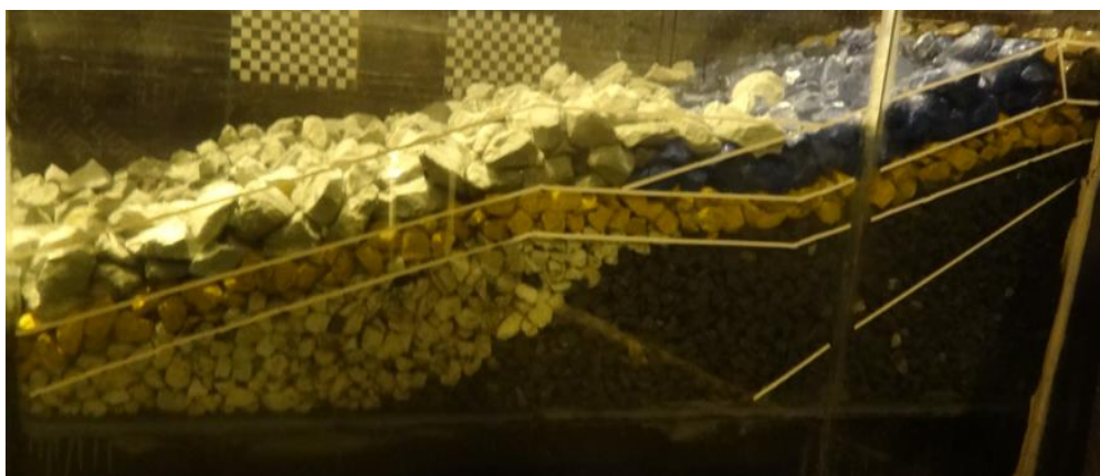
Figure 4.6 View of Section 1 after Set 3 (7000 waves)
