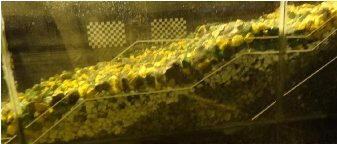
Figure 4.29 View of Section 4 after set 3 (8000 waves)
