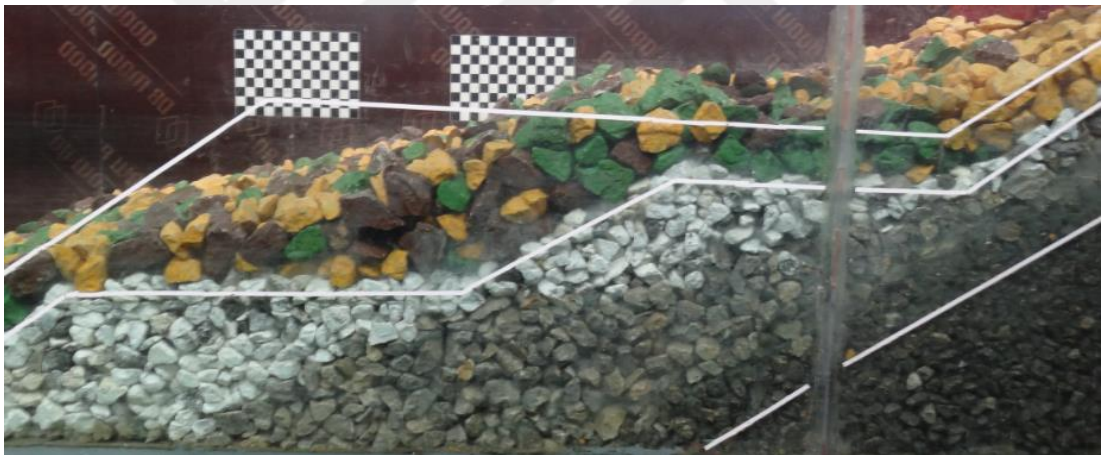
Figure 4.28 View of Section 4 after set 3 (4000 waves)
