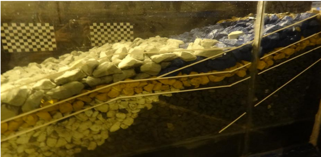
Figure 4.2 View of Section 1 after Set 1 (1000 waves)
