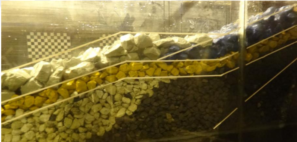
Figure 4.5 View of Section 1 after Set 3 (5000 waves)
