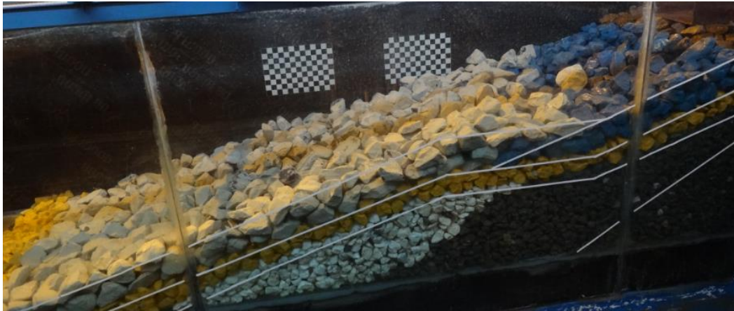
Figure 4.7 View of Section 1 after Set 3 (10000 waves)
