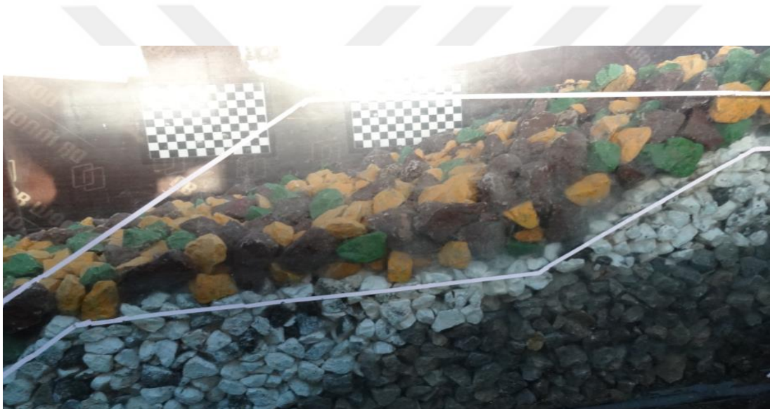
Figure 4.30 View of Section 4 after set 3 (10000 waves)
