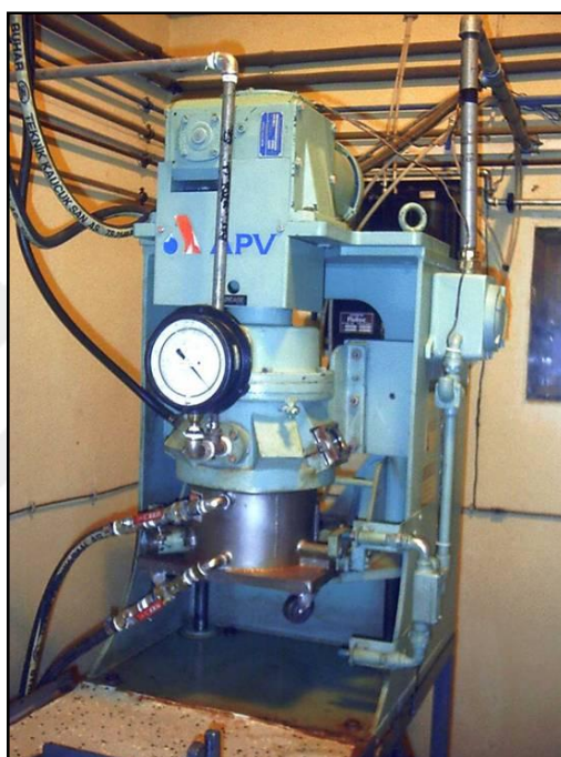
Figure 36 APV Baker 1 gallon mixer used in production of candidate propellant
