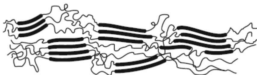
Figure 44 Schematic representation of a phase mixed polyurethane system [105].
