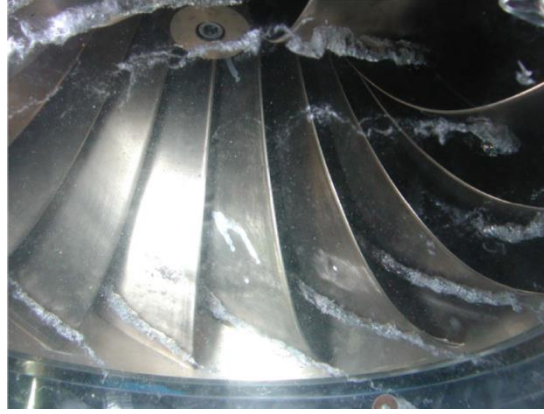
Figure 1.6 : Inter Blade Vortex
