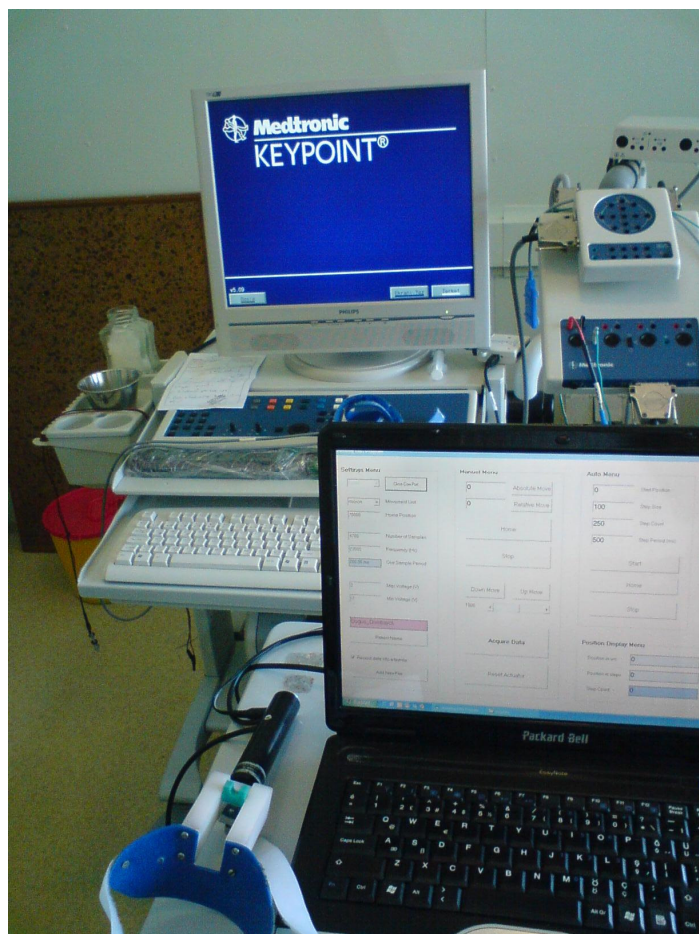
Figure 6.11 Experimental Setup of Scanning EMG connected to EMG instrument
