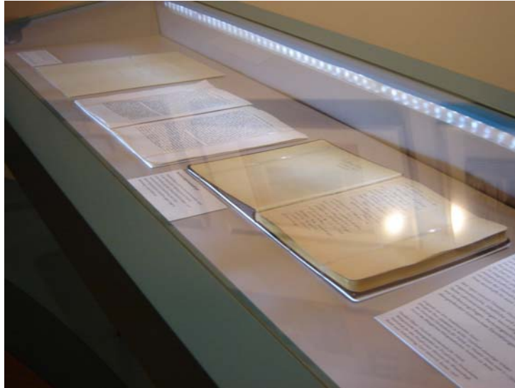
Figure 3.14 : Lighting of display cases causing reflections on the glass surface at Theodor Heuss Museum (Photo taken by Şener, F., 2007)
