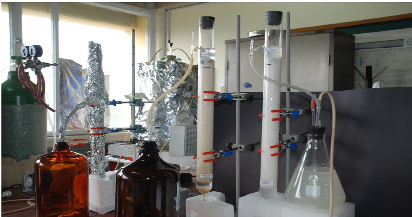
Figure 3.12. The general view of the the biological denitrification columns.
