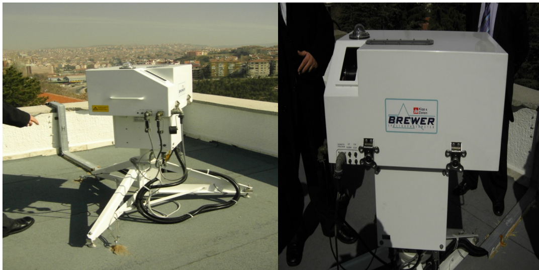
Figure 3.5: Brewer MK III Spectrophotometer
