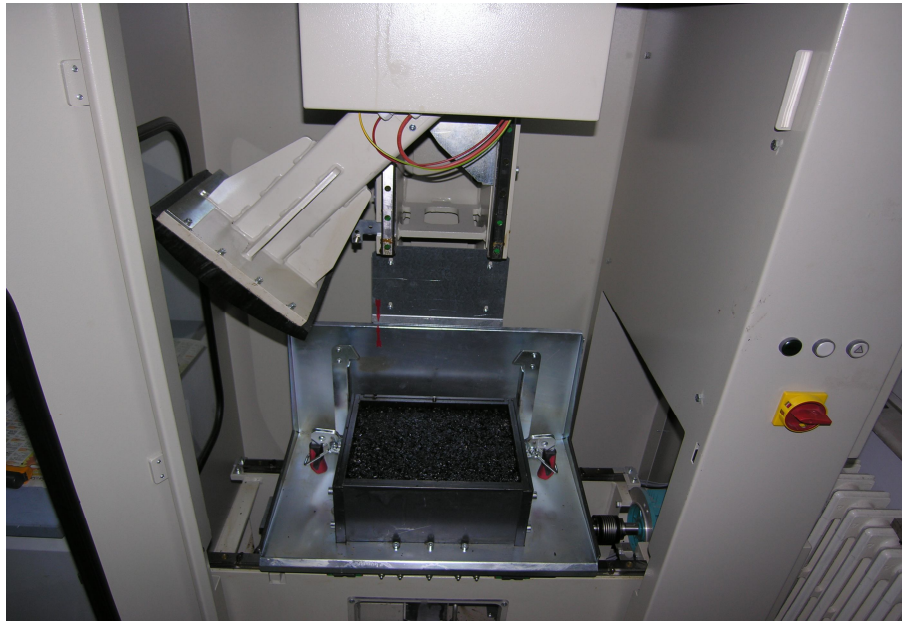
Figure 6.9. Compaction of slabs in segmental compactor.
