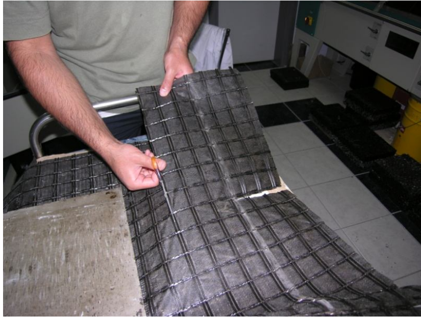
Figure 6.6. Preparation of geosynthetics for test: Cutting of material
