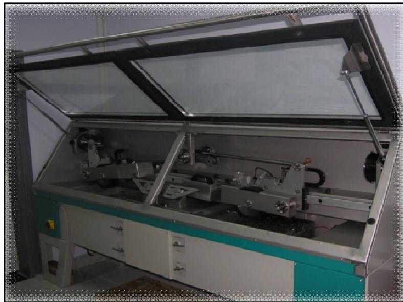
Figure 6.11. A Hamburg Wheel Tracking Device
