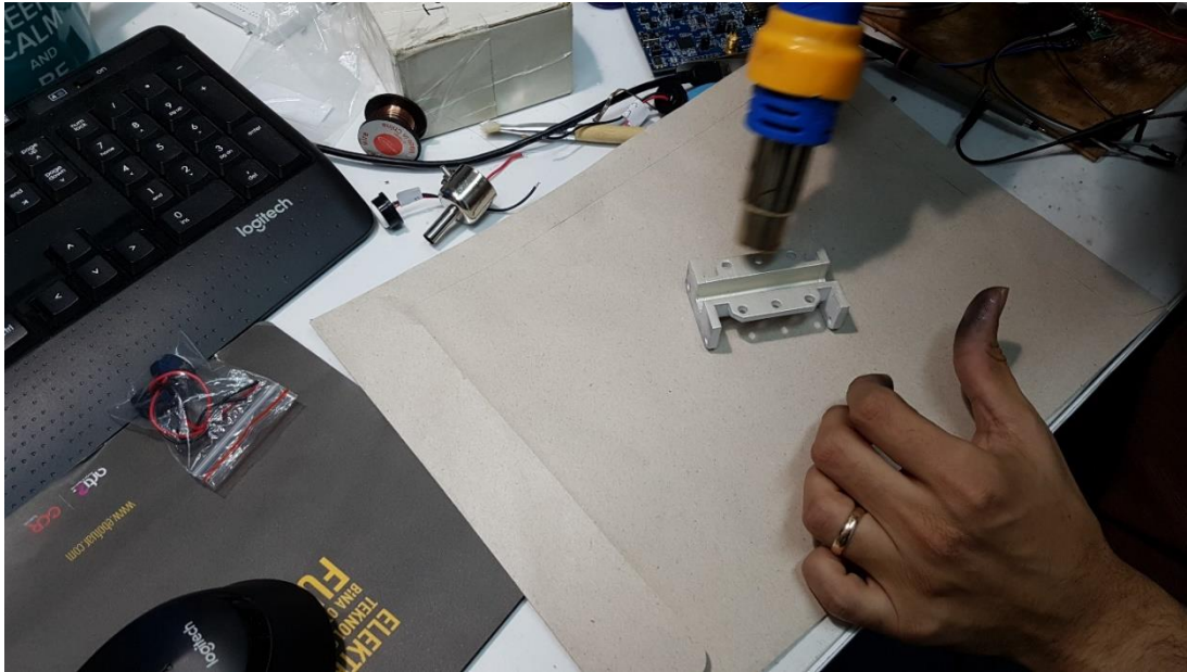
Figure 4.14: Curing the paint with heat gun
