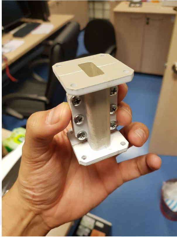
Figure 4.16: Final form of waveguide test piece
