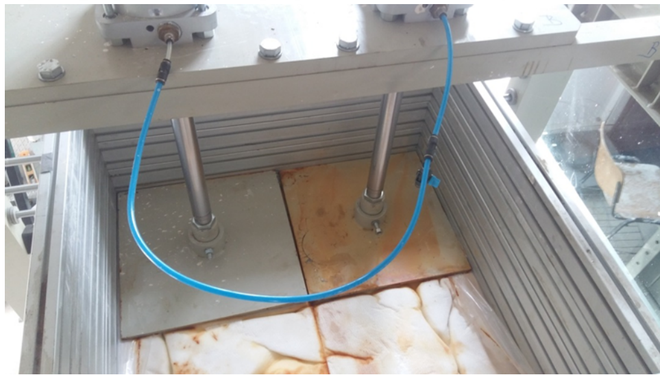
Figure 4.8. Two of the surcharge plates.
