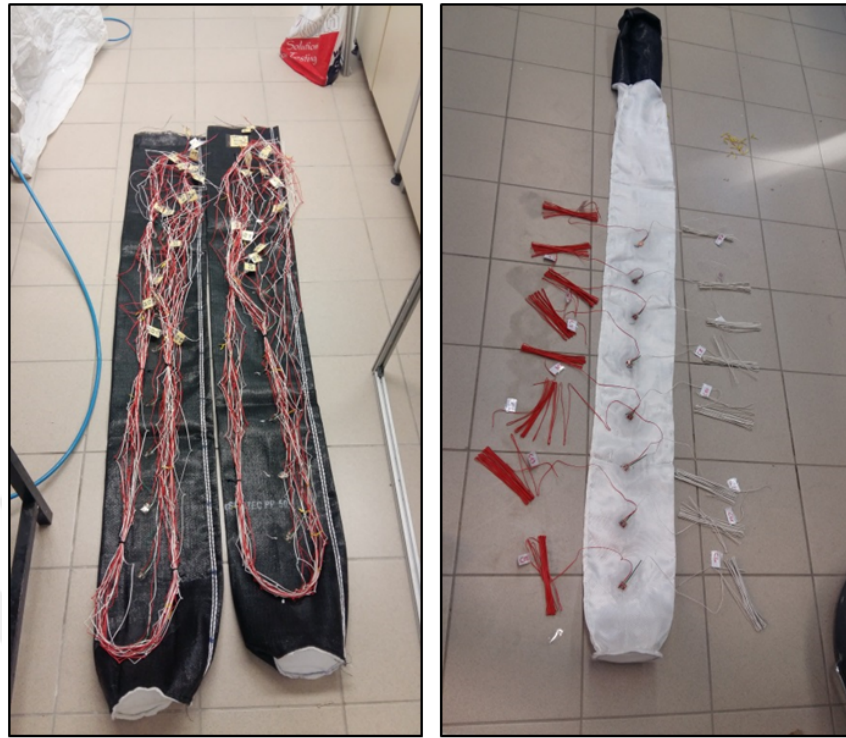
Figure 4.21. Instrumented reinforcements made up of GT2 and GT3.
