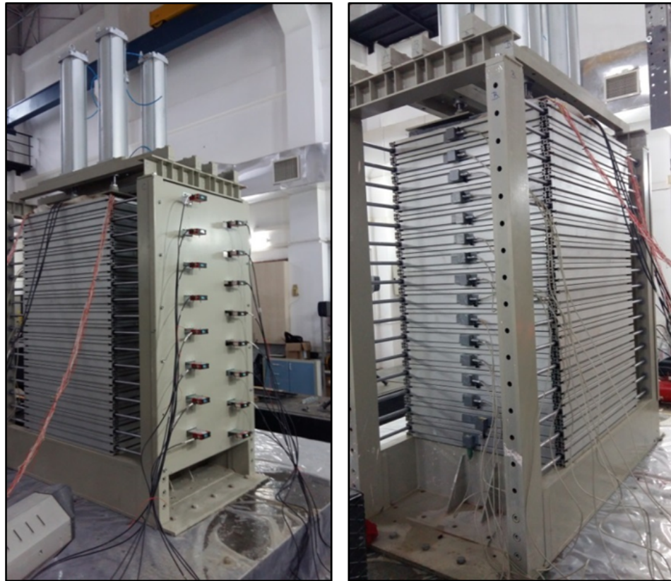
Figure 4.11. Laser displacement sensors and accelerometers attached on the laminar box.
