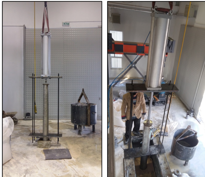
Figure 4.4. Casing pipe driving unit.
