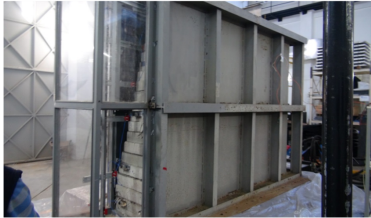
Figure 4.1. The rigid box assembly used by Kilic (2014).
