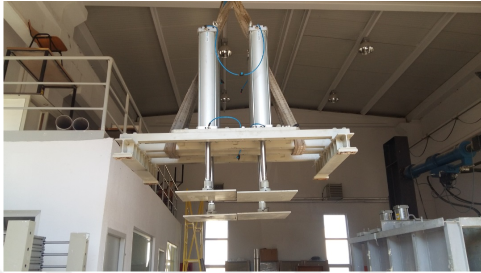
Figure 4.9. The surcharge unit suspended in the air.
