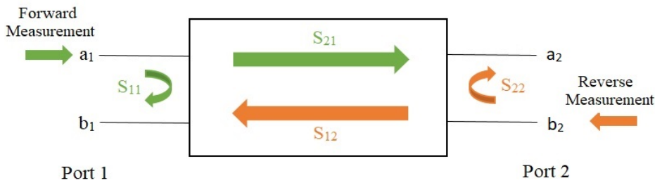
Figure 5.2 : Representation of the ports and scattering parameters in a 2-port VNA
