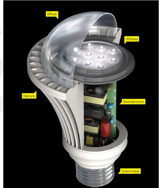
Figure 1.7 Schematic of an LED bulb. Image courtesy [21].
