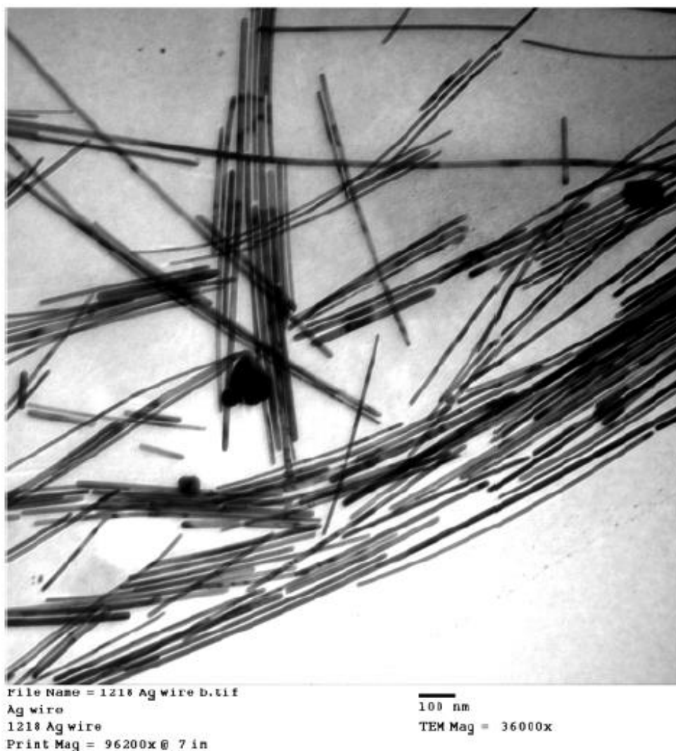
Figure 2.4 TEM image of shape-separated Ag NWs synthesized through seed-mediated approach [40].
