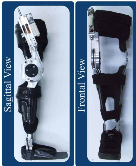
Figure 1.16. Quasi-passive compliant stance control orthosis lateral and frontal of prototype [19].
