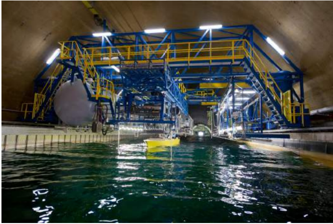
(c) A ship being towed using a crane rail system along the basin.
