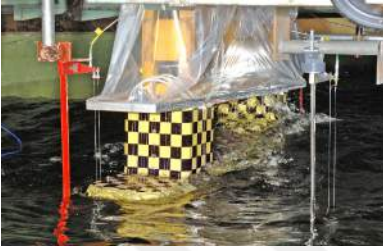
(a) A semi-submersible model whose position is fixed at the test section of the wave basin.
