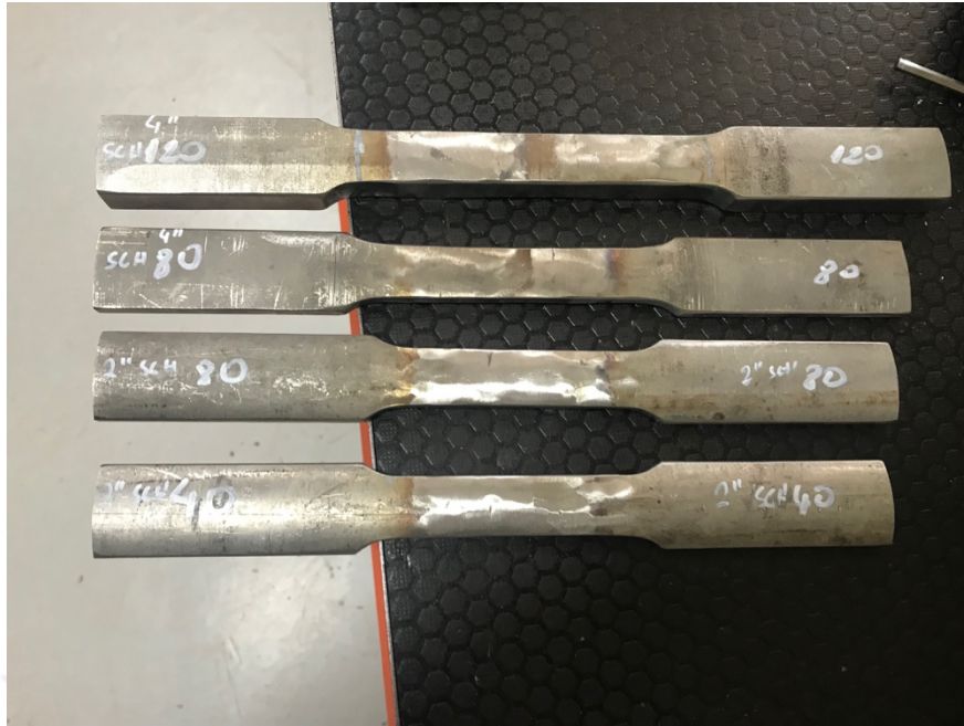
Figure 4.4: Tensile test samples.
