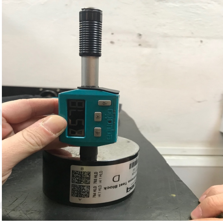
Figure 4.3: PROCEQ Equotip Bambino 2 Portable Hardness tester collibration.
