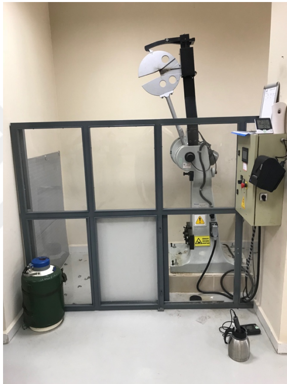
Figure 4.9: ASLA 450J Impact Test Machine.
