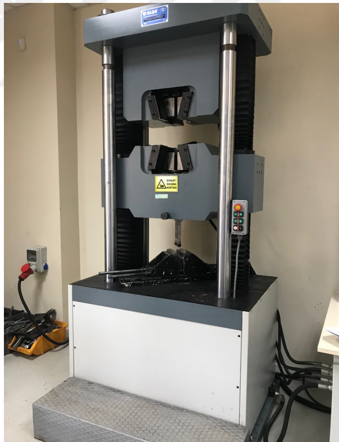
Figure 4.5: ASLA Universal Tensile Test Machine.
