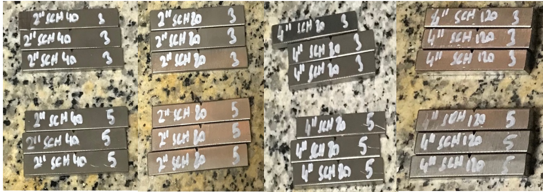
Figure 4.8: Prepared Charpy Impact Test samples
