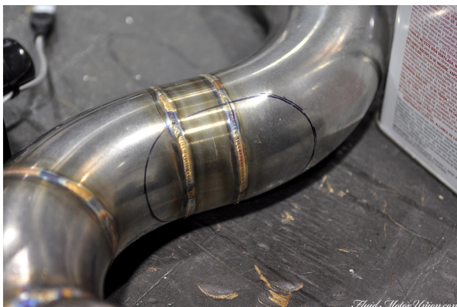
Figure 1.1: two close welds [1]
