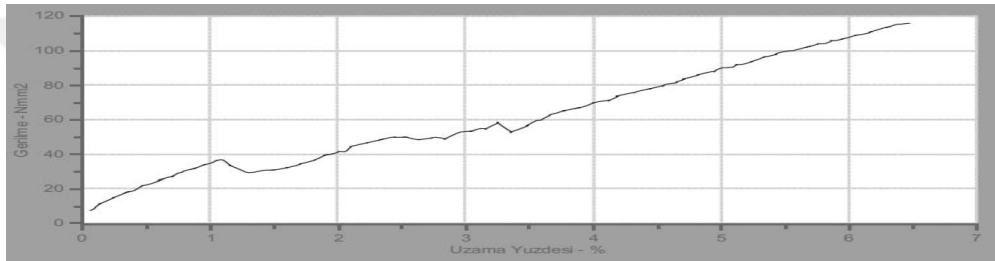
Figure 5.18. Stress-Strain results of third sample of the JGBA Composite ( \epsilon (%):6,5, \sigma_m :115,86 MPa).
