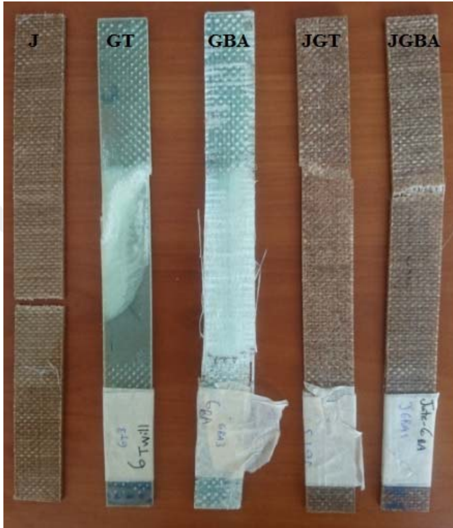
Figure 5.1. Tensile test specimens after the test.
