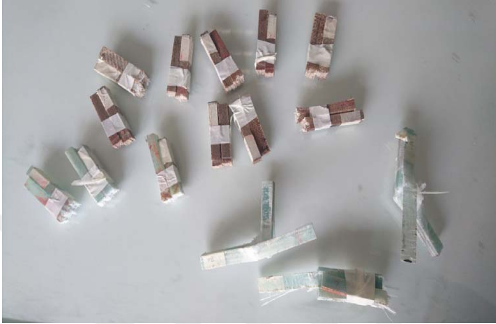
Figure 5.20. Charpy Impact Test Samples (After Test).
