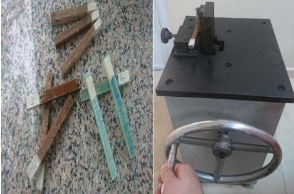
Figure 4.9. Notched Charpy Impact Test samples.
