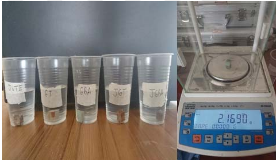
Figure 4.14. Water Absorption Test.
