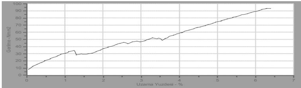
Figure 5.13. Stress-Strain results of first sample of the JGT Composite ( \epsilon(\%) :6,4, \sigma_m :93,29 MPa).
