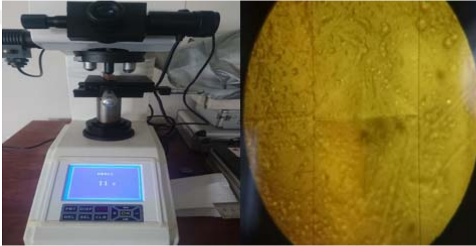
Figure 4.13. Vickers hardness Test and Pyramid Shaped Sample.
