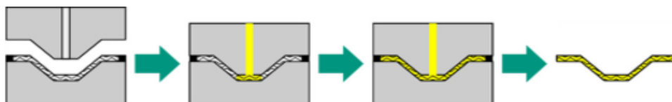
Figure 3.5. RTM process Flesicher J. et al., (2018).
