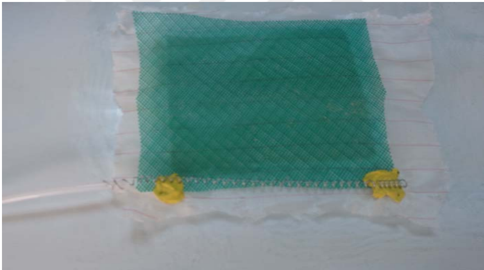
Figure 4.4. Infusion Filter on Peel Ply.
