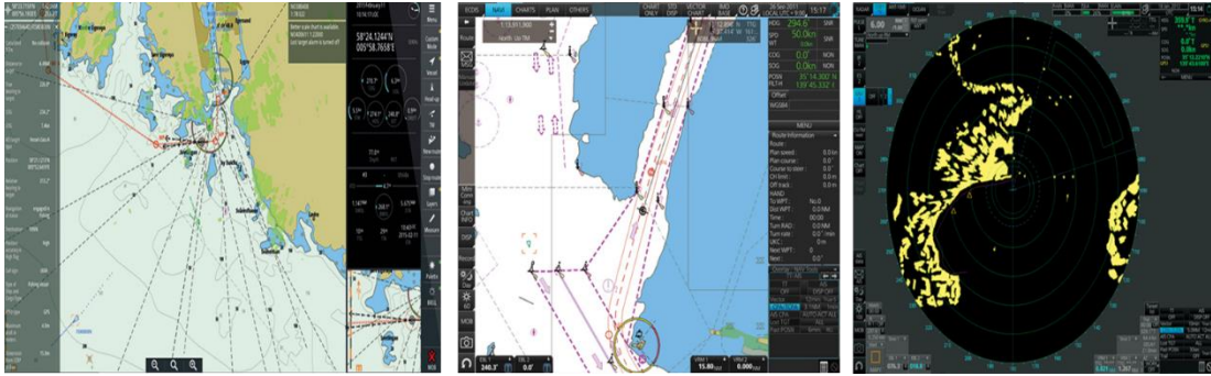
Figure 8. Different interfaces of ECDIS and Radar systems (Left to right: A Simrad ECDIS Interface, a Furuno display ECDIS Interface, a Furuno Radar Interface). Retrieved from [88], [89].
