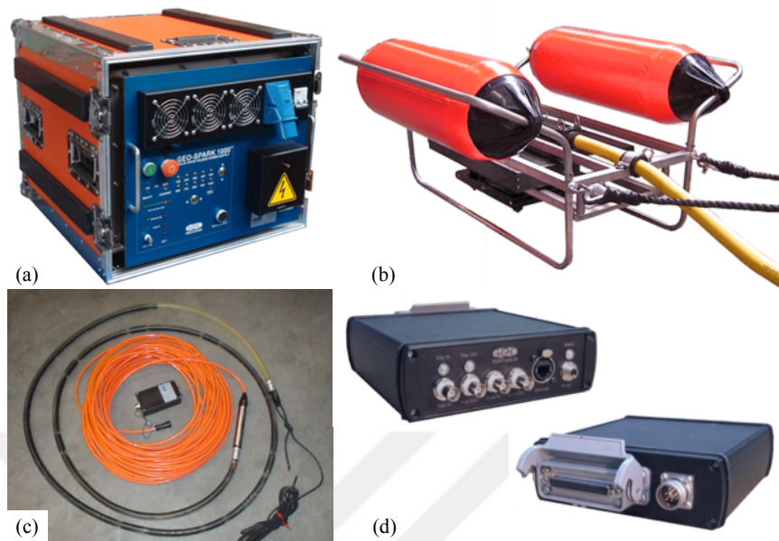
Figure 3.5 : Equipment used for data acquisition; (a) Geo-Spark 1000 Plus power supply, (b) Geo-Source Boomer Plate and catamaran, (c) Geo-Sense 8 Elements Mini-Streamer (AQ-2000 hydrophone) and (d) Multi-Trace II 24-bit double channel data acquisition system.
