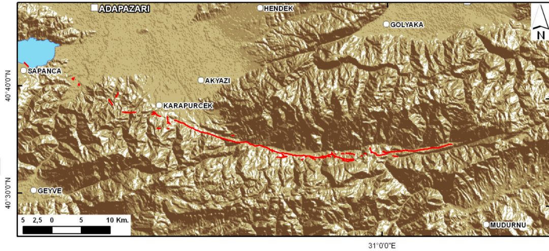
Figure 2.9 : Surface rupture of 22 July 1967 Mudurnu Valley earthquake (digitized from Ambraseys and Zapotek 1969) (Dikbaş, 2009).
