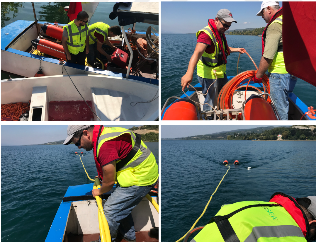
Figure 3.6 : Preparation and deployment of the boomer sub-bottom profiler equipment (SONARSEA).
