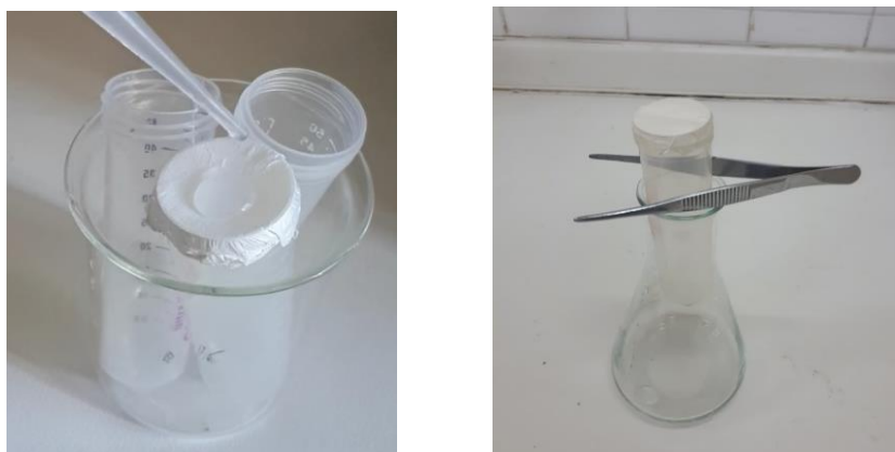
Figure 2.1: The image of the filtration process
