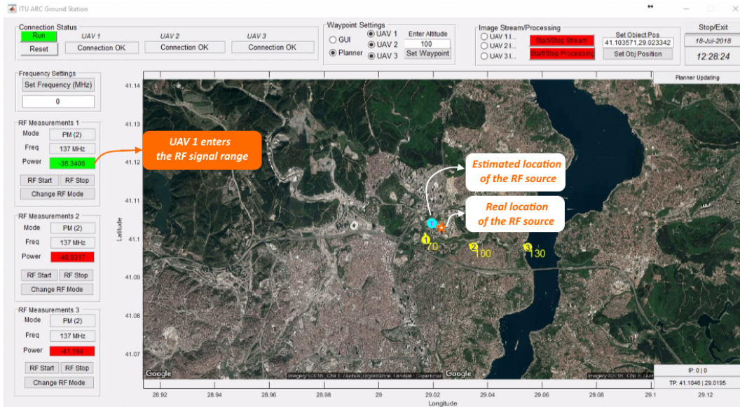
Figure 5.6 : An image of GUI screen when the first UAV measure the RF signal strength in the SIL testing.
