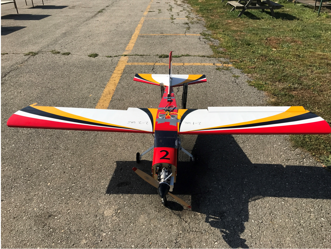
Figure 5.1 : The gasoline-engine UAV platform used in the tests.
