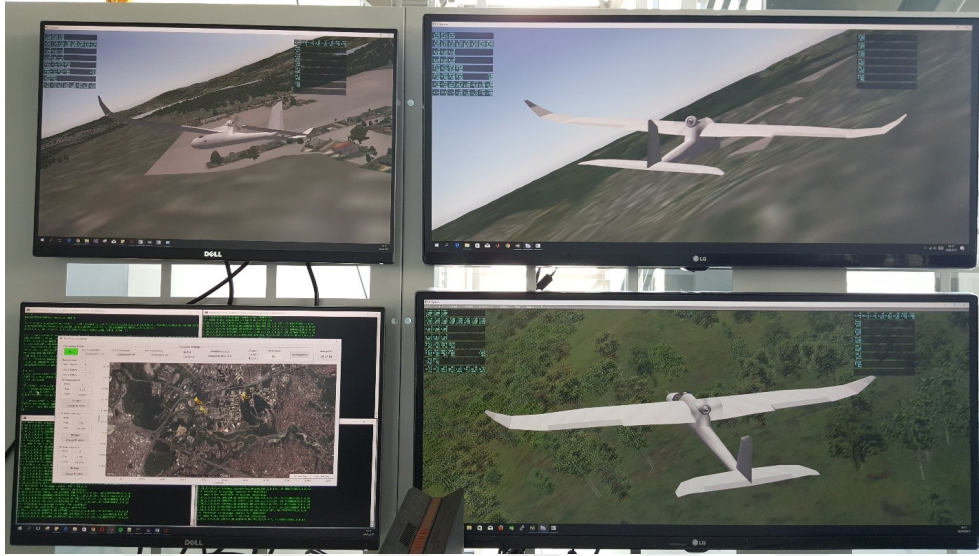
Figure 4.3 : An image of the SIL System Version I during a SIL test.
