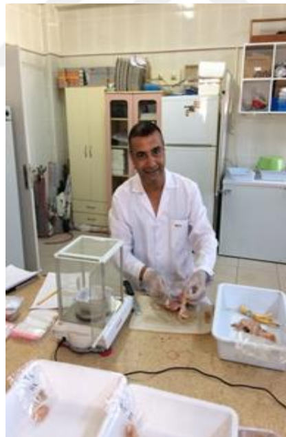
Figure 2.6. High precision balance (OHAUS max 410g- readability 0.001gm)
