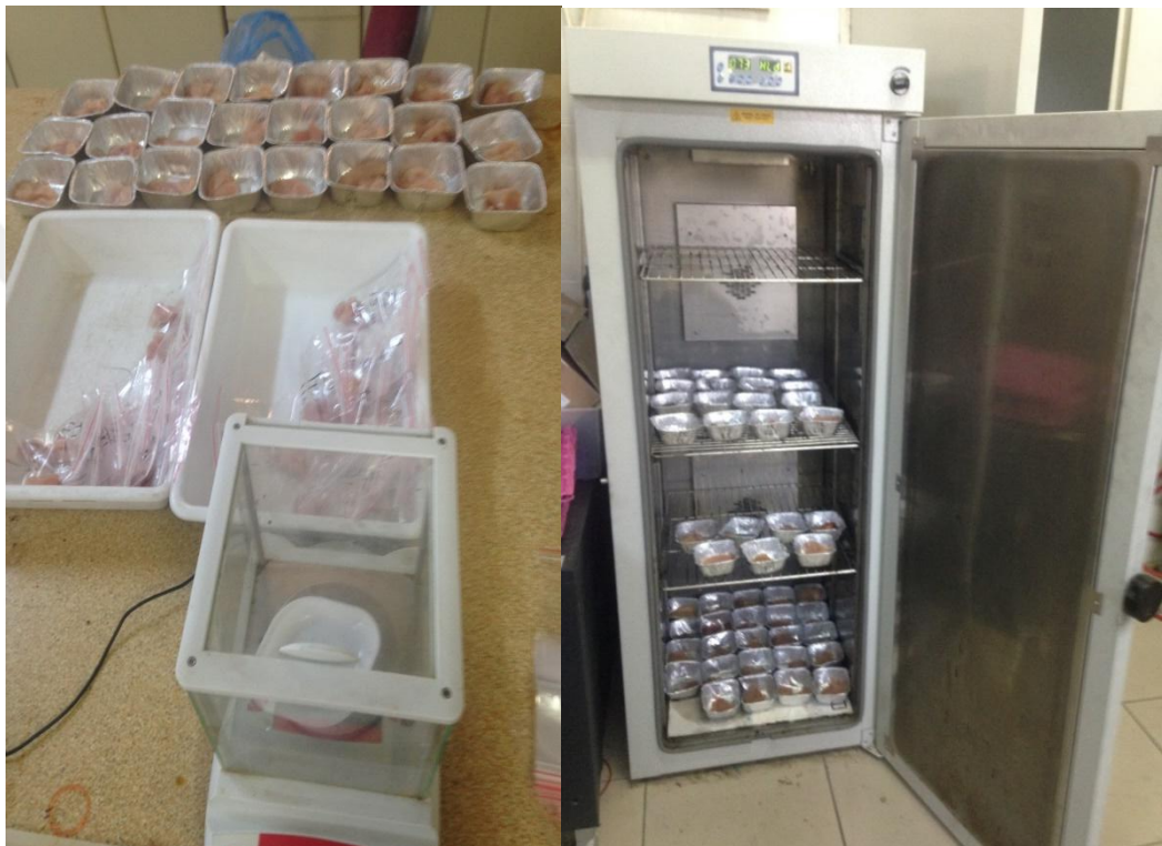
Figure 2.10. Laboratory oven (12 hours under the temperature of 105 °C)
