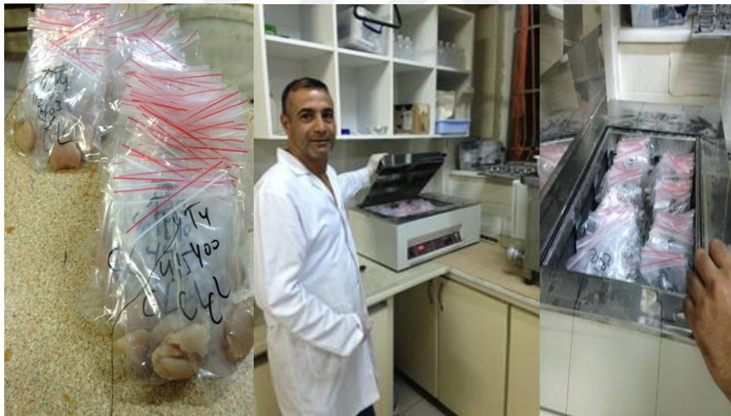
Figure 2.8. Cooking loss measurement (water bath GFL 1086)
