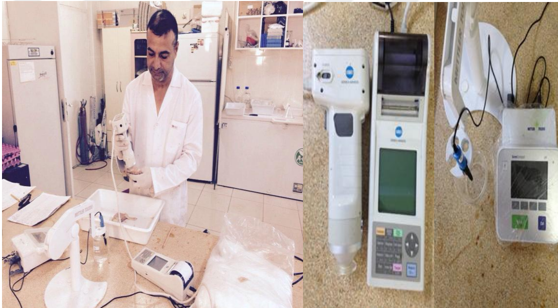
Figure 2.7. pH meter (Mettler Toledo- Swiss) and color detector Chroma-meter Minolta CR-400, Konica Minolta Sensing, Osaka, Japan
