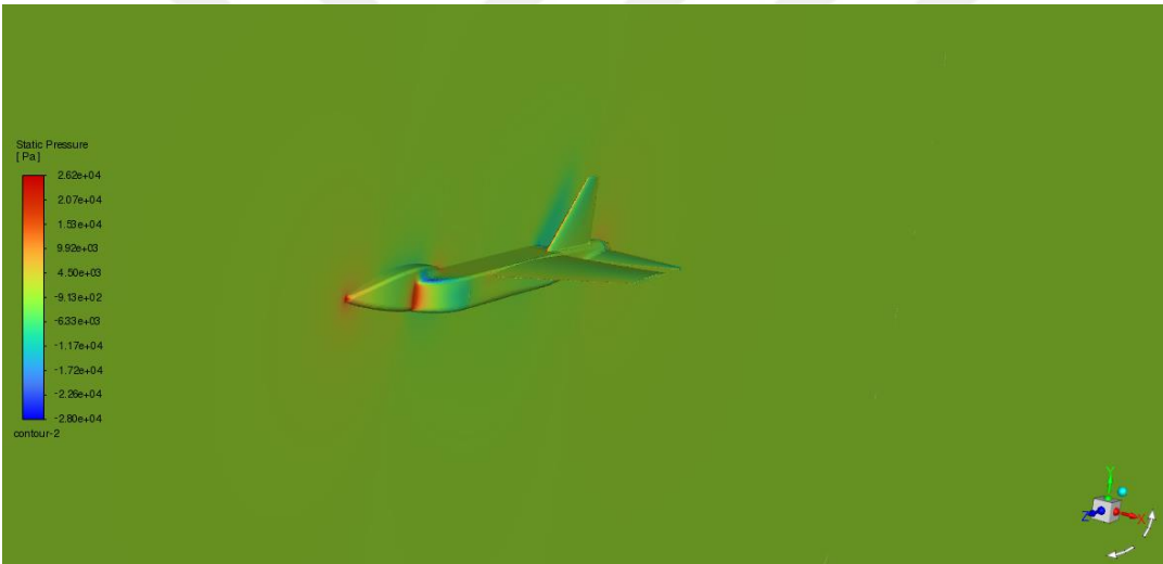
Figure 3.8: Contour of Static Pressure at M = 0.9 .
