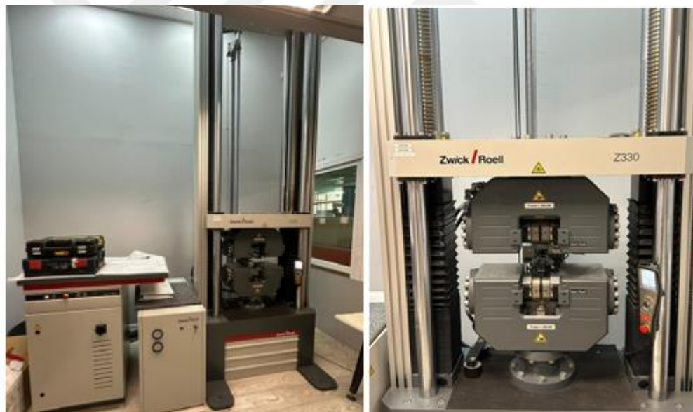
Figure 3.4 Modern closed-loop servo-hydraulic testing system (It was taken in Borcelik Testing Laboratories)
