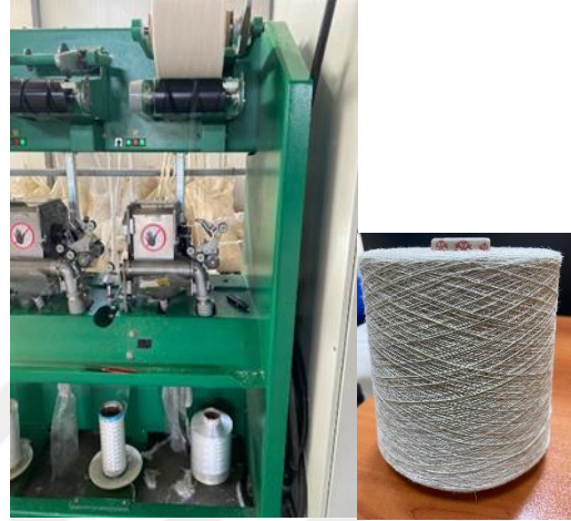
Figure 3. 2: Friction spinning machine and produced friction spun yarn.
