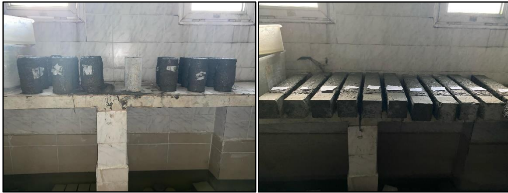
Figure 3. 25: Curing of reinforced cylinder and beam samples.
