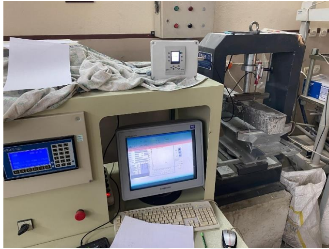
Figure 3.19: Flexural strength testing device.
