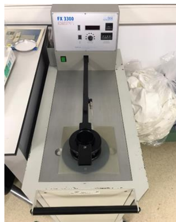
Figure 3. 16: Air permeability measuring device.
