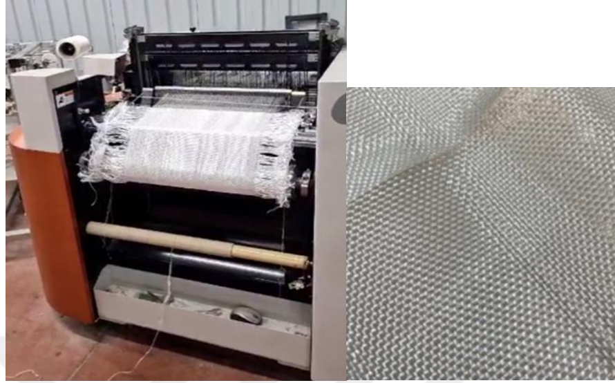
Figure 3.10: Woven fabric production with self-twisted Dyneema® yarn and the fabric produced.
