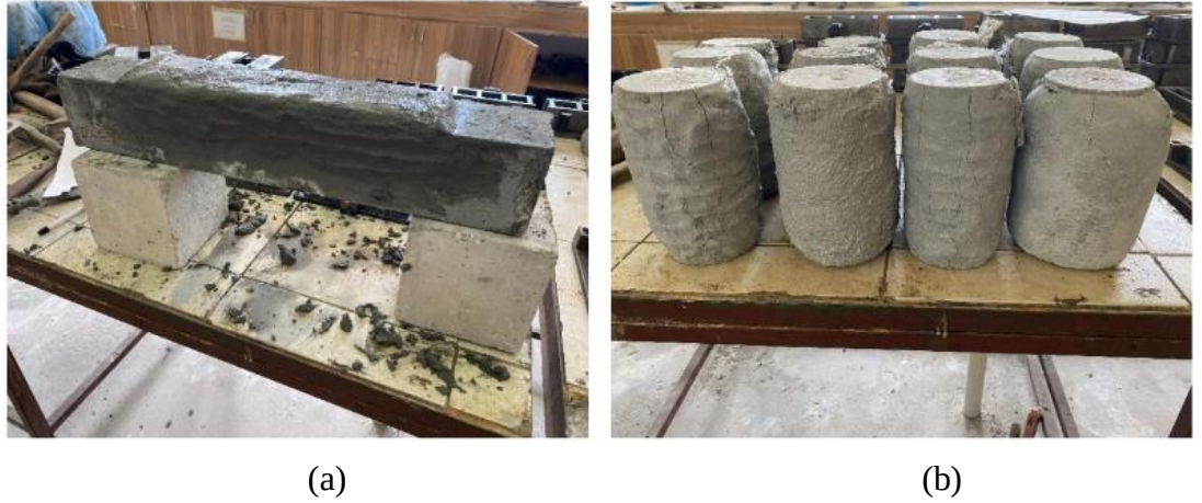
Figure 3. 24: Strengthening of beam specimens (a), strengthened and tested cylindrical specimens (b).
