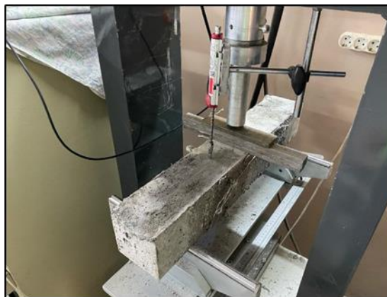
Figure 3. 27: Three-point bending test and deformation measurement applied to reinforced beam samples.
