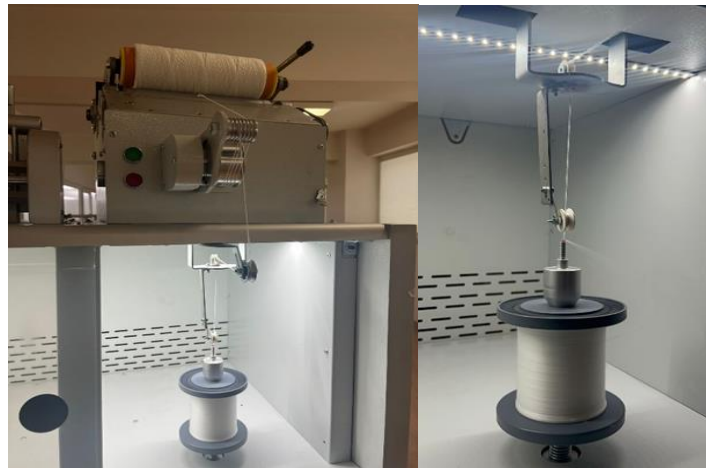
Figure 3. 8: Winding PVA yarn onto Dyneema® yarn.
