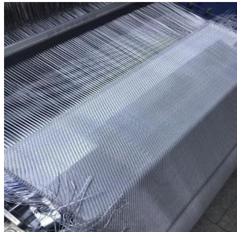
Figure 3. 5: Production of dyneema® yarn twill fabric.
