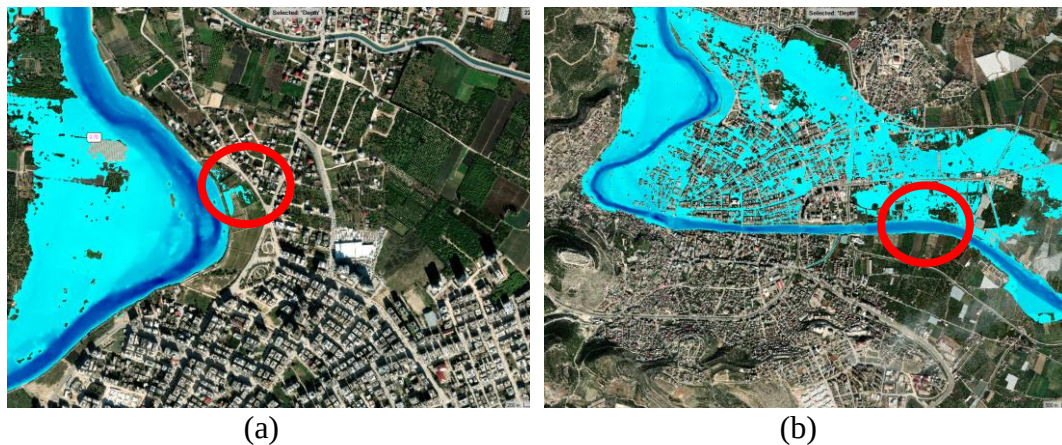
Figure 6. The combined 1D/2D coupled hydraulic model results: (a) The entering location of flood water (b) The leaving location of flood water (Basemap source: Esri, Maxar, Earthstar Geographics, and the GIS User Community)
