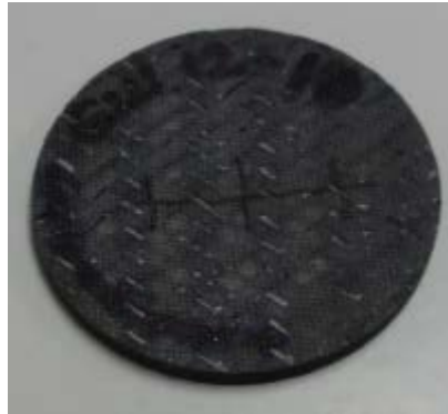
Figure 4.37 Representative transversely loaded specimen showing no visible damage.
